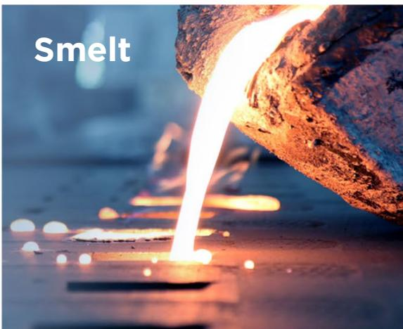
Heat at ultra high temperature to melt the Rare Earth Cerium and Magnesium metals.
