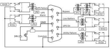
Fig 2 Connection for ACTIVE CLOSE
