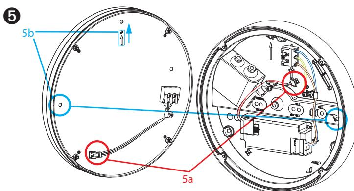
5a Connection of LEDs / 5b Position of diffuser
