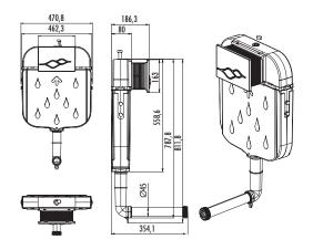
h (height) indicates the drift axis from the completed floor and it is approximately 320 mm. However the absolute measurement should be adjusted in accordance with the drift of the closet to be used.
