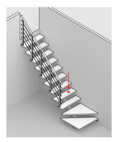
STAIR POINT LOAD Max. 2 kN ~ 200 kg
