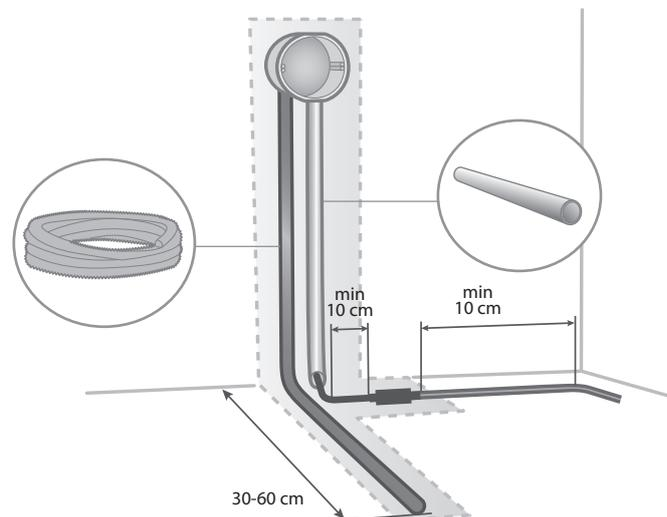
2a. The underfloor heating cable has a 3.0 metre connection cable. Put this into a plastic pipe designed for electrical material (not included in the Thermoflex Kit). *With the supplementary kit, both cables should be pulled up and connected in parallel in the thermostat.*
