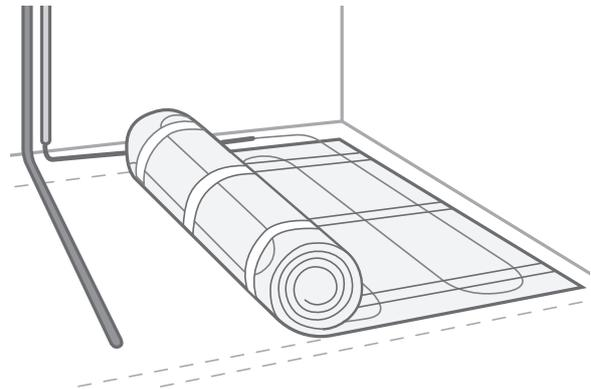
4. Roll out the matting to the opposite wall. Cut the mesh without damaging the cable. Roll the matting back again. The cables should not be closer than 5 cm to each other when cutting the mesh.
