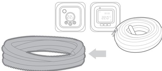
1b. The end of the sensor cable must not be covered by mats or fittings.
