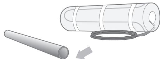
2b. The splices for the connection cable and the end terminal must not be placed in or next to any shower room or floor drain.
