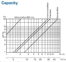
The lines for the filter alternatives illustrate fully open vent.
