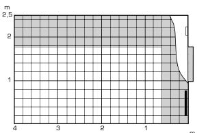
Outdoor temperature ±0°C, indoor temperature +20°C. Airflow 10 I/s, capacity of radiator 400 W
