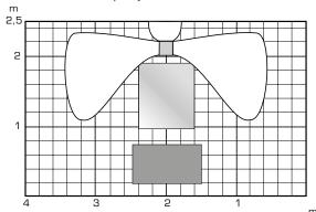
Outdoor temperature ±0°C, indoor temperature +20°C. Air flow 10 l/s, capacity of radiator 400 W
