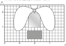
Outdoor temperature -20°C, indoor temperature +20°C. Air flow 10 I/s, capacity of radiator 400 W
