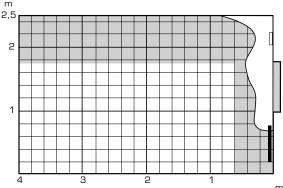
Outdoor temperature -20°C, indoor temperature +20°C. Air flow 10 I/s, capacity of radiator 400 W
