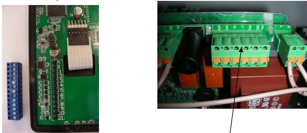
Connecting terminal markers A, B, 11 and 12 of the Control panel T2
