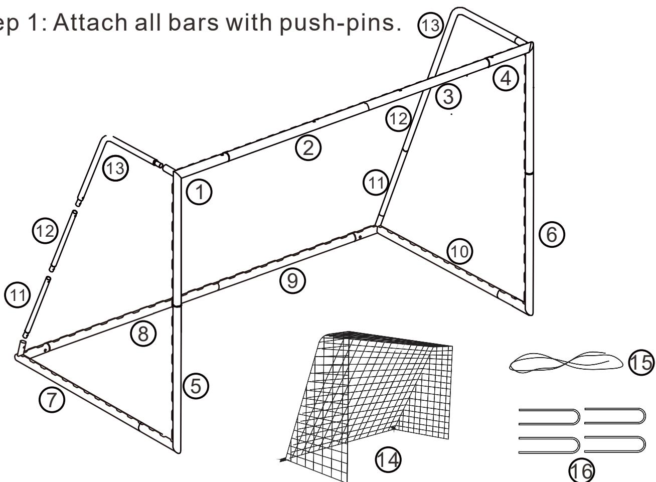
Step 2: Attach the goal net #14 to welded loop with rope #15.
