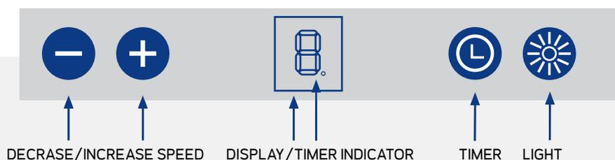
When the appliance is connected to mains power source, the operational mode of the appliance must be set to X1 (within 1 minute of connecting to mains current) by pressing the and keys simultaneously for at least 4 seconds. After, press the or keys until number 1 (= X1 mode chosen) appears on the display. Save the X1 mode by pressing the timer key . The operational mode of the appliance can be re-set by disconnecting and re-connecting the appliance to mains current.
