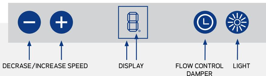
When the appliance is connected to mains power source, the operational mode of the appliance must be set to X2 (within 1 minute of connecting to mains current) by pressing the and keys simultaneously for at least 4 seconds. After, press the or keys until number 2 (= X2 mode chosen) appears on the display. Save the X2 mode by pressing the The flow control damper key . The operational mode of the appliance can be re-set by disconnecting and re-connecting the appliance to mains current.
