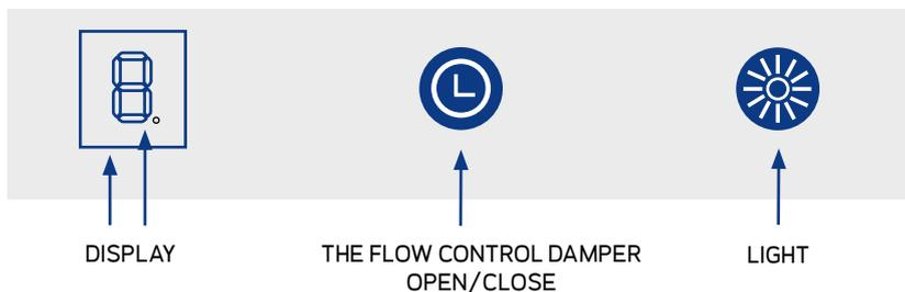
When the appliance is connected to mains power source, the operational mode of the appliance must be set to X3 (within 1 minute of connecting to mains current) by pressing the **-** and **+** keys simultaneously for at least 4 seconds. After, press the **-** or **+** keys until number 3 (= X3 mode chosen) appears on the display. Save the X3 mode by pressing the timer key **⌚**. The operational mode of the appliance can be re-set by disconnecting and reconnecting the appliance to mains current.
