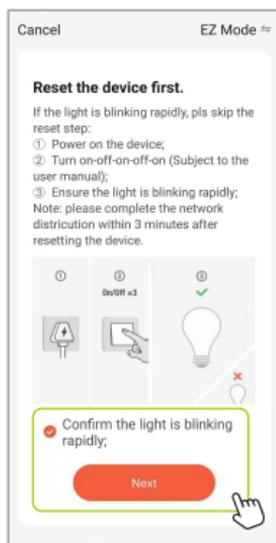
If you could see the rapid blinks from the connected fixtures, click “Confirm the light is blinking rapidly” → “Next”; If not, reset by turning Off/On by 3 times till it appears.
