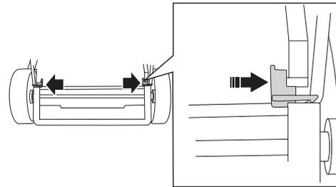
**IMPORTANT!** Both stop lugs for the handle must be assembled before the machine is used. Press in the lugs firmly.
