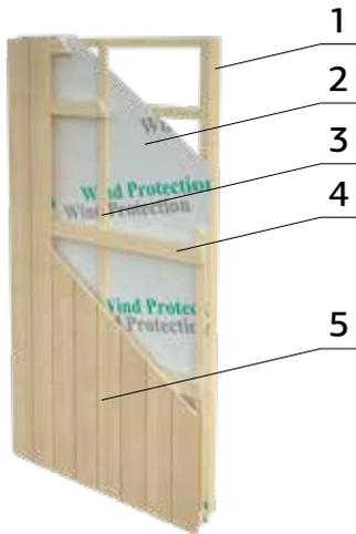
Total element thickness by Nordic+ houses is 160 mm. Here is a cross section of an element just to get a better understanding of what these elements look like and consist of:
