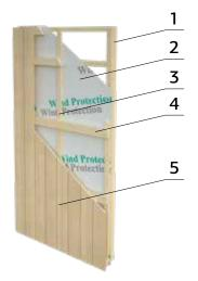
Total element thickness by Nordic+ houses is 160 mm. Here is a cross section of an element just to get a better understanding of what these elements look like and consist of:
