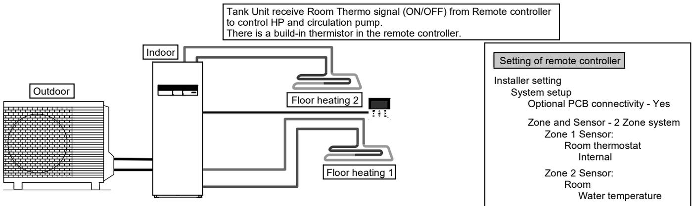
Connect floor heating or radiator directly to the Tank Unit.
