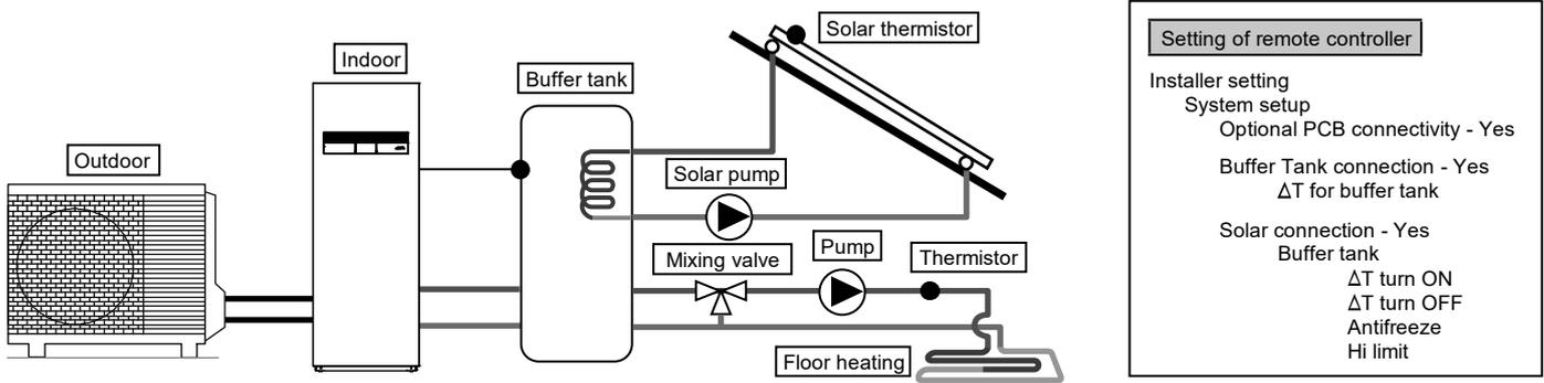
This is an application that connects the buffer tank to the Tank Unit before connecting to the solar water heater to heat up the tank.
