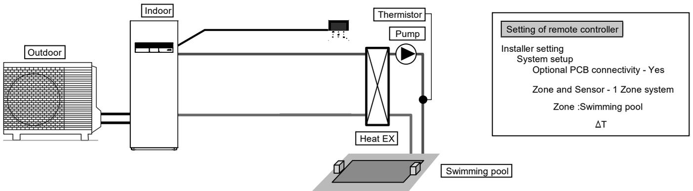
This is an application that connects to the swimming pool only. Connects pool heat exchanger directly to Tank Unit without using buffer tank. Install pool pump and pool sensor (specified by Panasonic) at secondary side of the pool heat exchanger. Remove remote controller from Tank Unit and install in room where floor heating is installed. Temperature of swimming pool can be set independently. This system requires the Optional PCB (CZ-NS5P).
