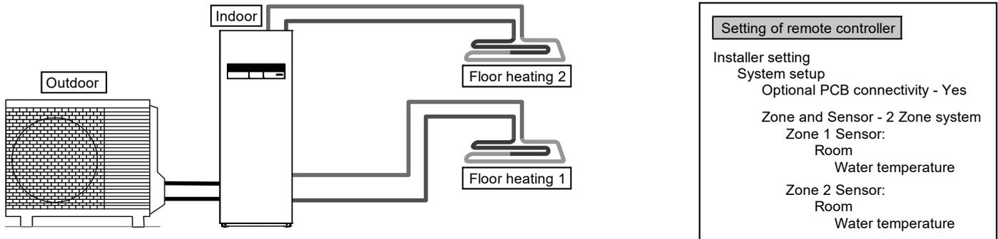
Connect floor heating or radiator directly to the Tank Unit.
