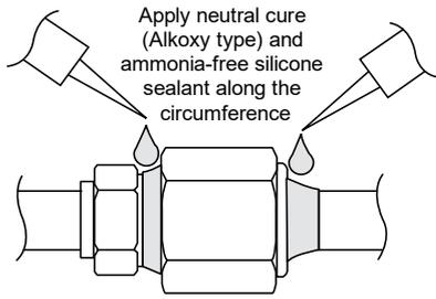
Neutral cure (Alkoxy type) & ammonia-free silicone sealant is only to be applied after pressure testing and cleaning up by following instructions of sealant, only to the outside of the connection. The aim is to prevent moisture from entering the connection joint and possible occurrence of freezing. Curing sealant will take some time. Make sure sealant will not peel off when wrapping the insulation.
