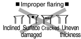
When properly flared, the internal surface of the flare will evenly shine and be of even thickness. Since the flare part comes into contact with the connections, carefully check the flare finish.
