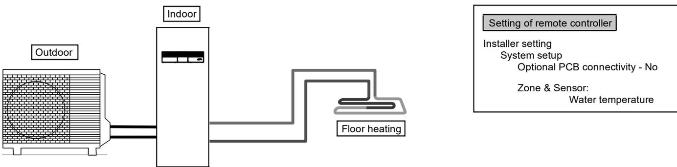
Connect floor heating or radiator directly to the Tank Unit.
