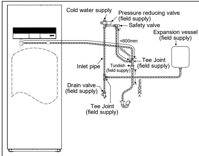
1. Connect the tundish and route the discharge pipe as shown above. Tundish should be visible and positioned away from frost environment and electrical components.
