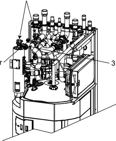
⚠ When reinstall Flow Switch, ensure the arrow on the flow switch is parallel with the pipe shaft and is facing in the direction of flow.
