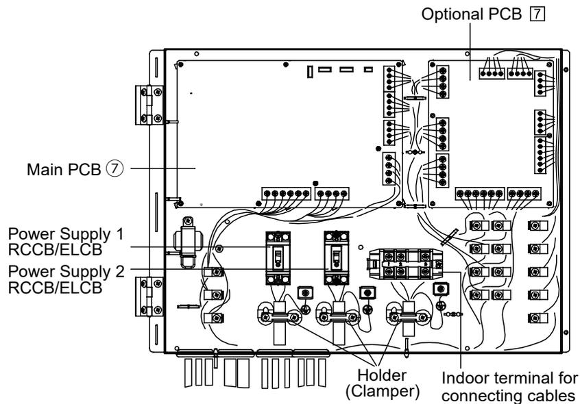
How to guide the optional cables and power supply cord
