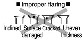
When properly flared, the internal surface of the flare will evenly shine and be of even thickness. Since the flare part comes into contact with the connections, carefully check the flare finish.
