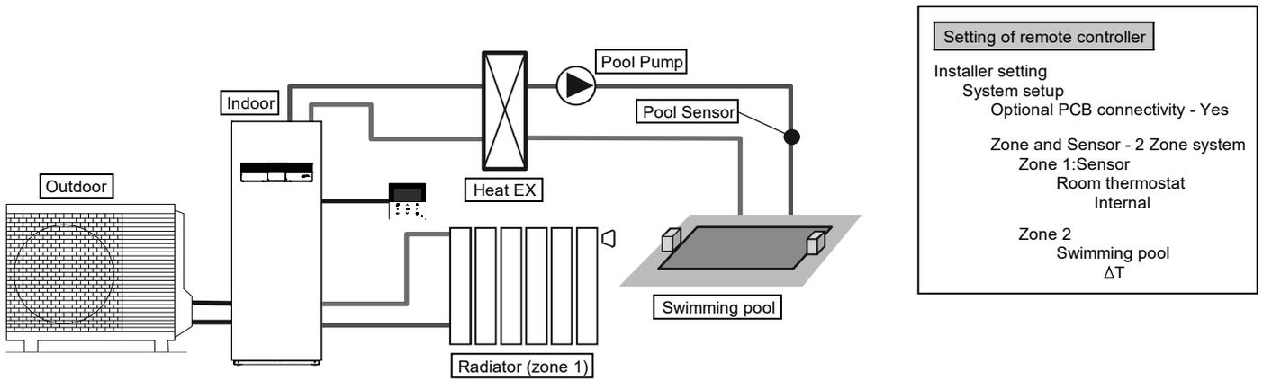
Connect floor heating and swimming pool to 2 circuits through buffer Tank Unit as shown in figure. Install additional pool heat exchanger, pool pump and pool sensor on pool circuit. Remove remote controller from Tank Unit and install in room where floor heating is installed. Circulation water temperature of floor heating and swimming pool can be set independently.
