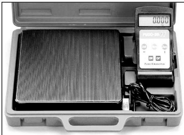
Digital scale for refrigerant charging
