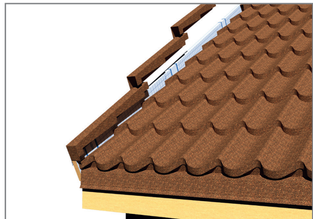
Fig 9.4.2 Gable flashing installation
