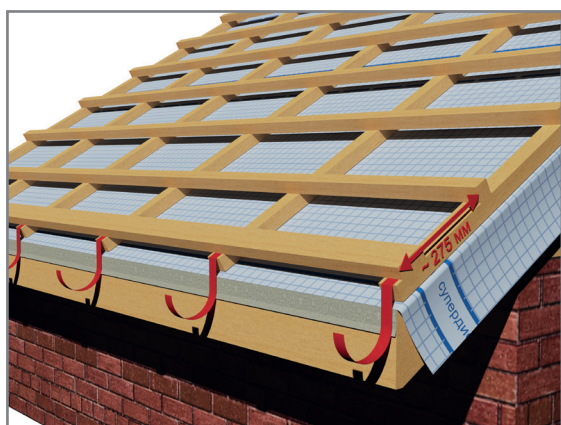
Fig 8.4.1 The roof sheathing with rainwater hooks
