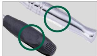
The obvious dent or electroplate desquamation indicates that a pipe wrench or hammer (or other form of "cheater") has been abused on this ratchet. Please use a larger size of ratchet to increase the leverage of any wrench.
