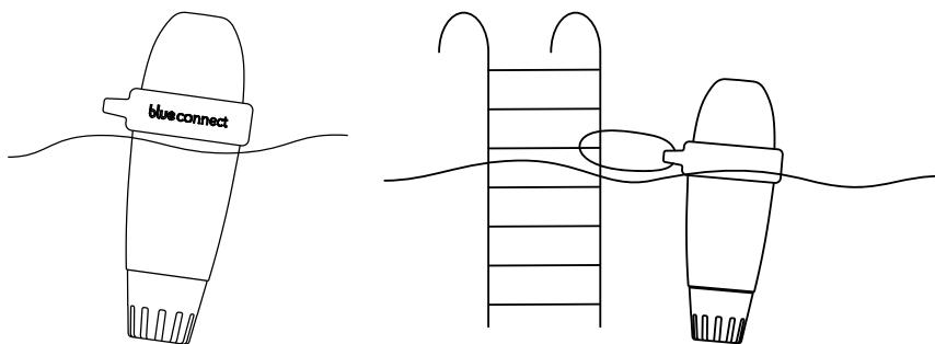
**NB:** Make sure the device is in vertical position and the top part out of the water to allow a correct communication.
