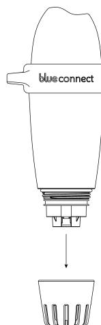
3. Wipe **Blue Connect** with a clean, absorbent cloth, paying special attention to properly drying the bottom part of the product (where the probe is located) without touching the sensors.
