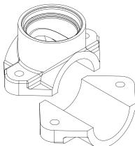
**Blue Fit50**: The hose clamp for installing **Blue Connect** on the technical room pipes (see p.17)<sup>3</sup>.
