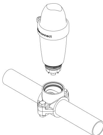
**2.** Seal the hose clamp with the cap provided in the **Blue Fit50** box.
