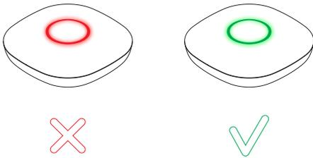
6. To verify if the Blue Extender is well positioned and not too far from the Blue Connect, press on the button of the Blue Extender casing.
