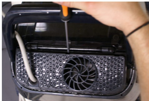
7.1. Use a flat screwdriver to remove the protective grille.
