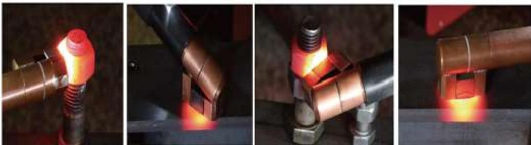
Heating a rusted nut so that it can be quickly and easily removed from machinery, cars, etc. Using thermal expansion theory, heating a rusted nut causes it to expand, making it easier to remove. Similarly, heating the glass of a car makes it easier to remove it from the car.
