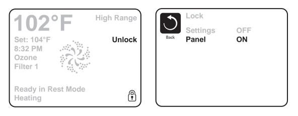
An Unlock Sequence using the navigation buttons can be used from the Lock Screen. The Unlock Sequence is the same for both Panel Lock and Settings Lock.
