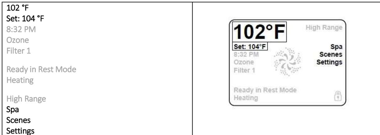
The only main display option that can be changed in the left edge of the main display is the preset temperature. Touch the preset temperature line or water temperature option to navigate to the preset temperature display.
