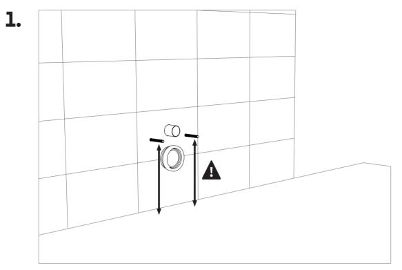
Please note, that the installation requires a pre-installed concealed cistern that must comply with standard EN 14055:2010. Leave enough space between the floor to tighten the bolts.
